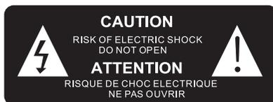
The lightning symbol inside an equilateral triangle warns the user of the presence inside the product of uninsulated hazardous electric voltages powerful enough to represent an electrocution risk.
